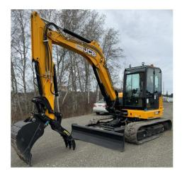
This JCB 86-C Excavator weighs 19,000 lbs. It has 24 feet of digging reach, 18 feet of dump height, heated and cooled cab and a highquality stereo system so you can move lots of dirt in comfort.
